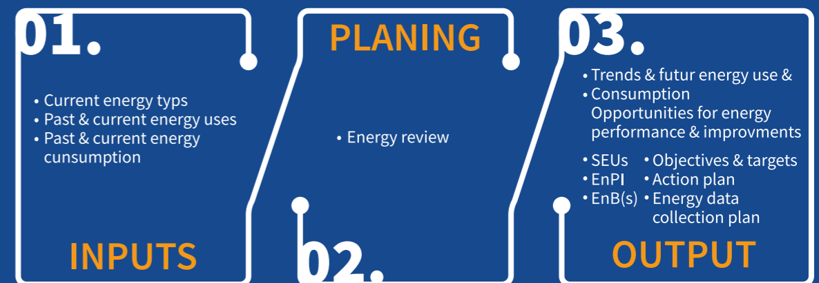
Figure 1 : Key main stages in energy planning starts with energy data collection and then followed by the energy review that will produce the planning outputs.
